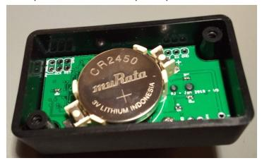
• When replacing the back cover make sure the foam on the cover is aligned with the battery. This prevents the battery from becoming dislodged from the battery holder during use.
