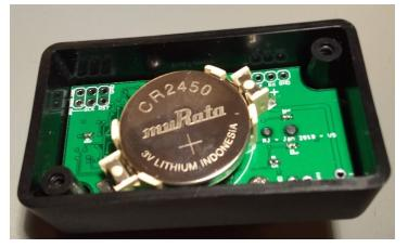
• When replacing the back cover make sure the foam on the cover is aligned with the battery. This prevents the battery from becoming dislodged from the battery holder during use.
